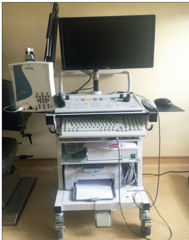
Figure 3 Natus Nicolet device - registers the electrical activity of the brain during electrical stimulation of the olfactory mucosa
