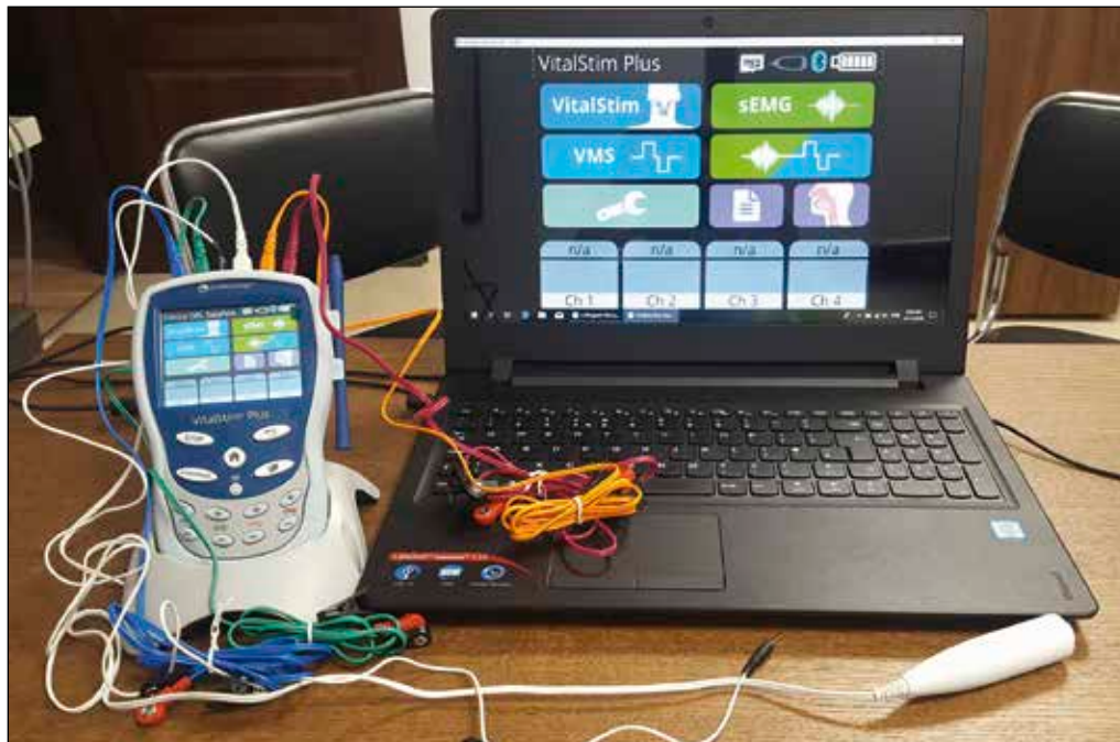
Figure 1 VitalStim® Plus Electrotherapy System (Chattanooga Group, Chattanooga, TN, USA), a 2-channel surface electromyography (sEMG) and 4-channel electrotherapy.
