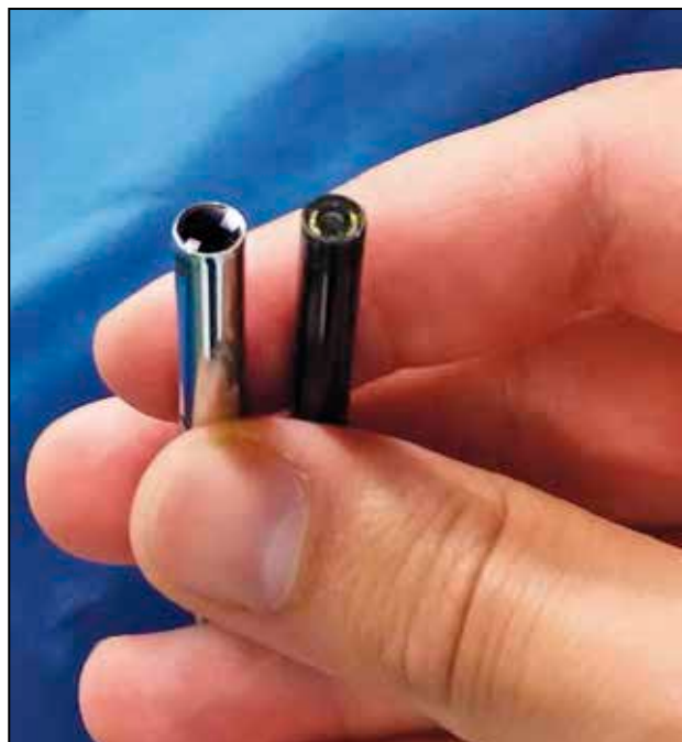
Figure 2 Inner and outer part of the prototype endoscope. The outer part is a metal tube, ending with a 0° lens.
