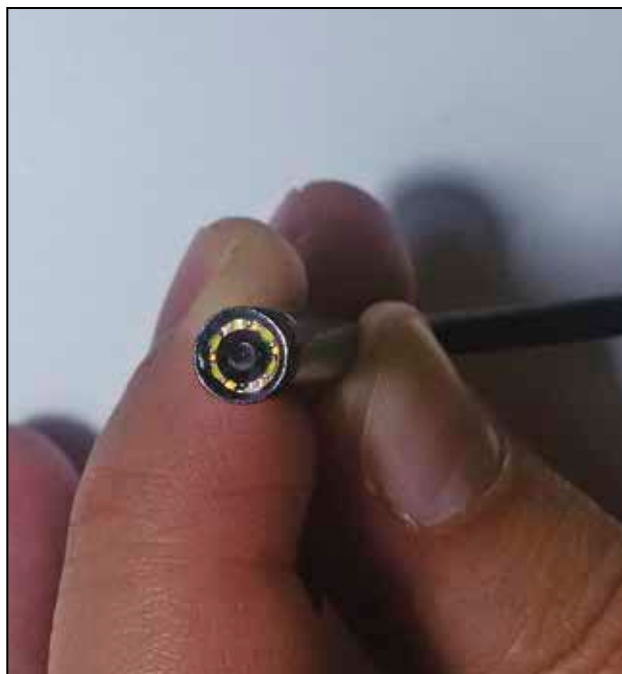
Figure 1 The inner part of the rigid chip-on-the-tip endoscope, consisting of chip-on-the-tip low-cost camera with 6 micro LEDs for illumination.
