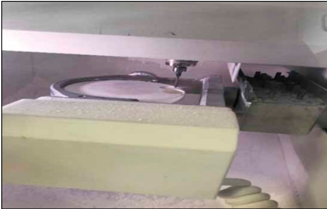
Figure 12. Computerized milling of copings in a zirconium dioxide disc.
