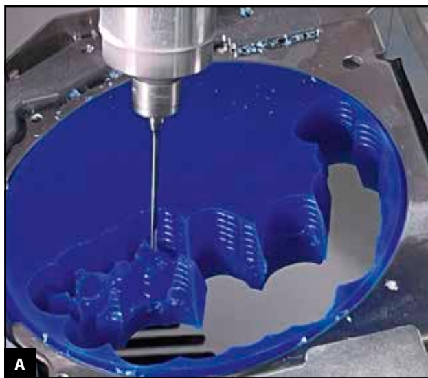
Figure 5. The aspect of the wax pattern of the metallic component of prosthetic restoration while milling (A) and at the end of the milling process (B).
