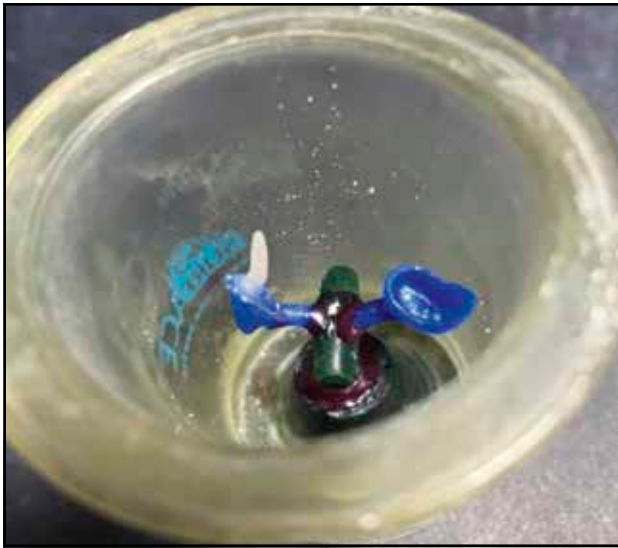
Figure 13. The silicone cylinder is attached to the crucible former cone to check the distance between the wax pattern and the walls of the cylinder.
