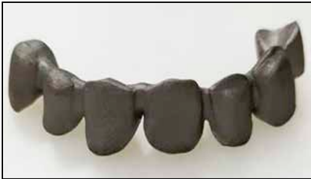
Figure 5. Metal substructure obtained after computerized milling.
