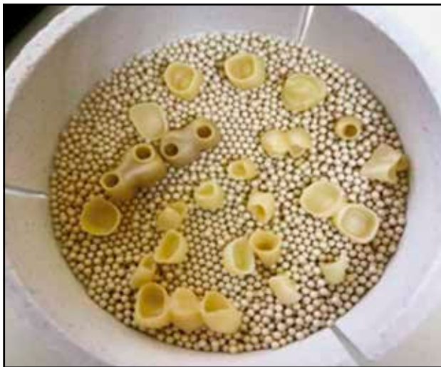
Figure 6. Zirconia copings at the end of the sintering process.
