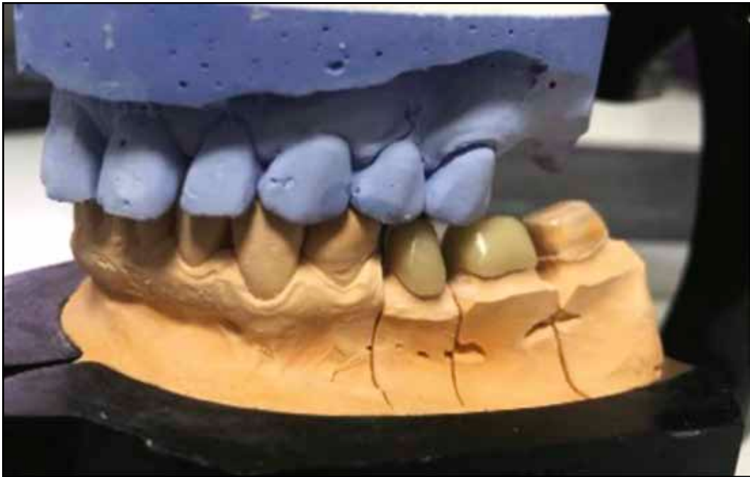
Figure 13. Zirconia copings on the functional model, before being sent to the dental office for try-in.
