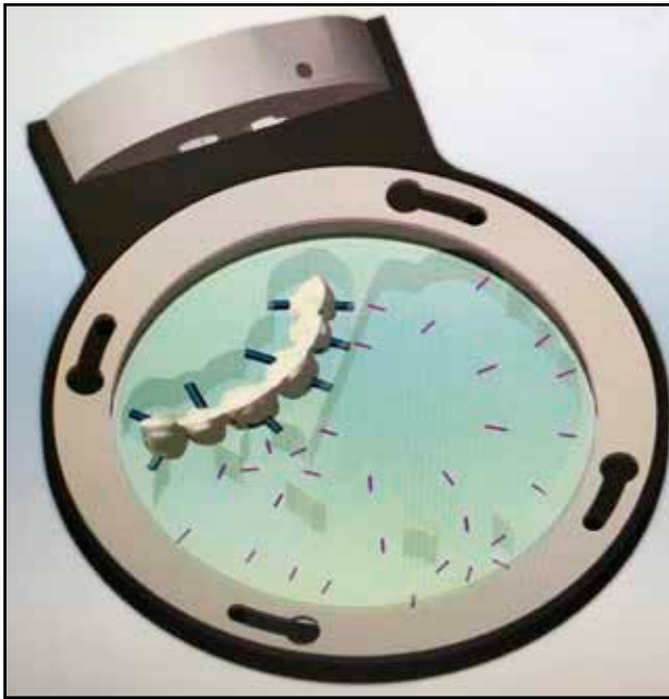
Figure 5. The virtual image of substructure is positioned on the virtual image of zirconia disk.
