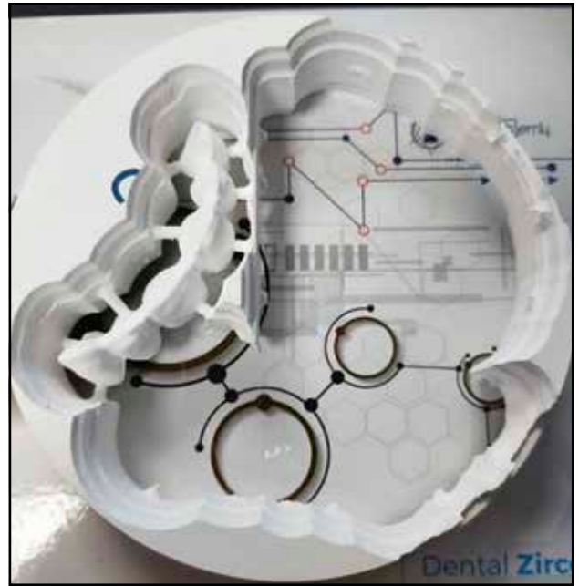
Figure 6. The zirconia substructure at the end of the milling process.
